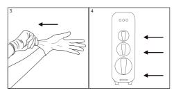
· To sanitize the equipment, the filters must be inside their housings (4).
