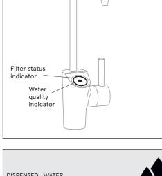
BLUE: right TDS in dispensed water. DISPENSED WATER MAGENTA: medium TDS QUALITY in dispensed water. RED: high TDS in dispensed water. BLUE / MAGENTA / RED Blinking indicator while **FLUSHING** the unit is flushing the membrane. **BLINKING BLUE** BLUE: working properly. MAGENTA: a mainte-FILTER LIFESPAN nance will be required **STATUS** soon. RED: the spanlife of some filter has expired. BLUE / MAGENTA / RED
