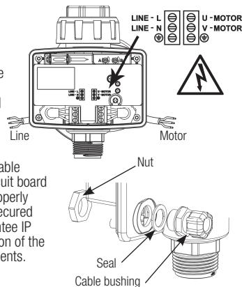
**Attention!** The cable bushings and circuit board cover must be properly assembled and secured in order to guarantee IP 65 grade protection of the electrical components.
