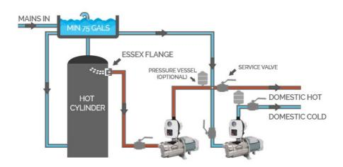
\*Double Check Valves should be installed on hot and cold supply pipes before all points where 'cross over' between hot and cold supplies can occur, such as mixer taps and mixer showers.
